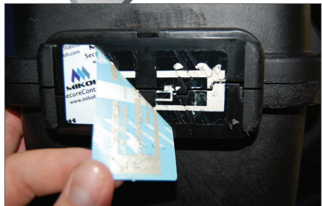
Figure 1 | A tamper-evident RFID tag in the process of being destroyed during a tamper event
