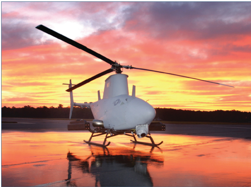
Figure 2 | Vertical Takeoff and Landing Tactical UAVs (VTUAVs) can take off and land in rugged or unimproved terrain in close proximity to troop and tactical operations centers. Acting as a communications node within the Joint Tactical Radio System (JTRS), they extend both network effectiveness and flexibility.
